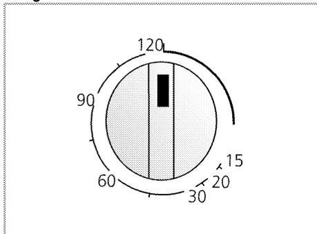
The alarm clock has no influence on the functions of the oven. It is only used as a warning. For example, this is useful when you want to turn food in the oven at a certain point of time. Alarm clock will give a signal once the time you set is over.
