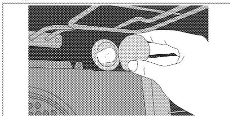
3. Remove the oven lamp by turning it counter clockwise and replace it with the new one.
