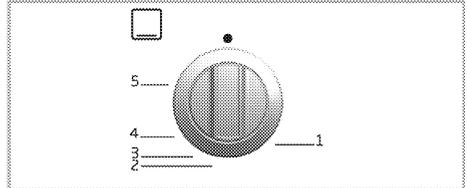
The gas oven is operated by the gas oven control knob. In off position (top) the gas supply is Off.
