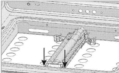
5. Remove the oven burner from housing.
