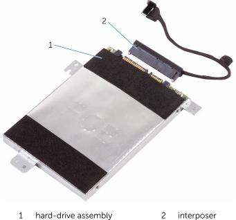
Remove the screws that secure the hard-drive bracket to the hard drive. 7
