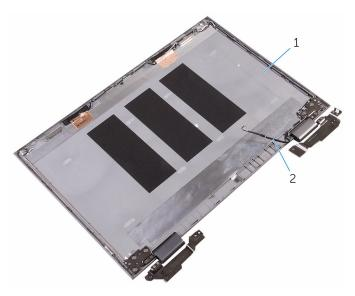
display back-cover and antenna 2 antenna cables assembly
