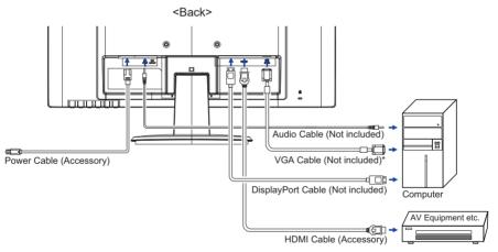
\* VGA cable is not supplied with the monitor. If you use low quality VGA cable, it may cause a result of electro-magnetic interference. Please contact the iiyama Support Centre in your country if you wish to connect the monitor via the VGA input. Signal Timing
