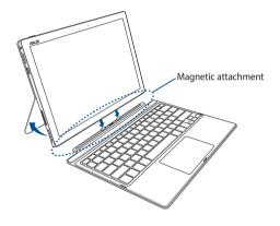
**WARNING!** Keep the magnetic attachment away from external storage drives and cards with magnetic strips to prevent demagnetization.
