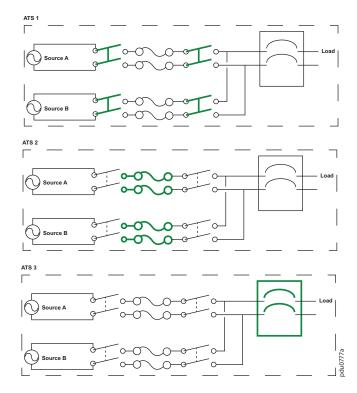
The rack ATS does not include power surge protection. To protect your ATS from external power surges, it is always recommended that you connect each ATS source to a Double Conversion On-Line Uninterruptible Power Supply (UPS).
