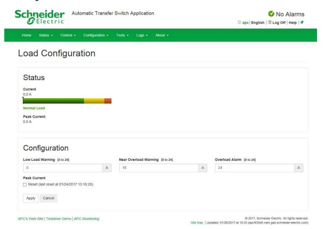
**Status:** View the current in A, and the Peak Current in kVA, for the device, phases, and banks. The indicator in the green, yellow, and red meter shows the load status: normal, near overload, or overload.
