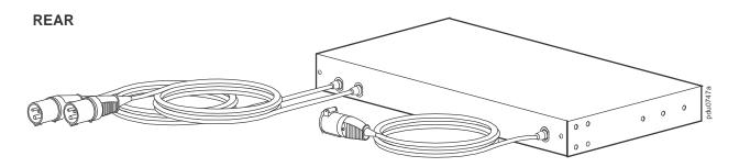
**Output Power cord:** The IEC 309-16A, 3-pin output cord connects the switch to a Rackmount PDU, providing a redundant source of power to the PDU and the equipment connected to it.
