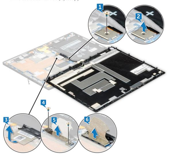
ONOTE: Only disconnect the display cable from the system board. DO NOT disconnect the display cable from the display panel.
