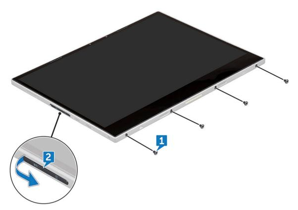
4 Insert a plastic scribe into the microSIM/microSD slot.
