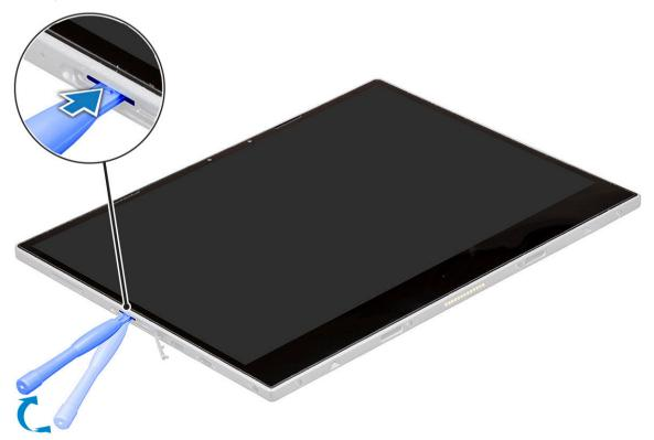
5 Pry the edges starting from microSIM/microSD slot [1, 2].
