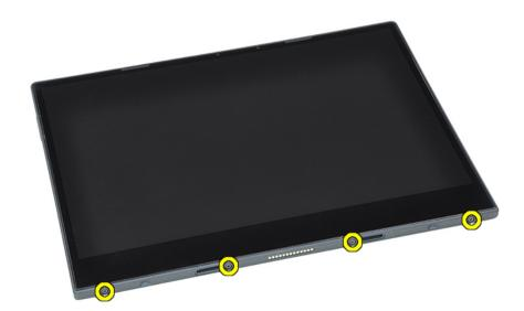
b Attach a suction cup to the display panel above the left docking slot, located at the bottom of the system, while inserting a plastic scribe into the left docking slot to stabilize the system, and then carefully pull open the display panel using the suction cup.
