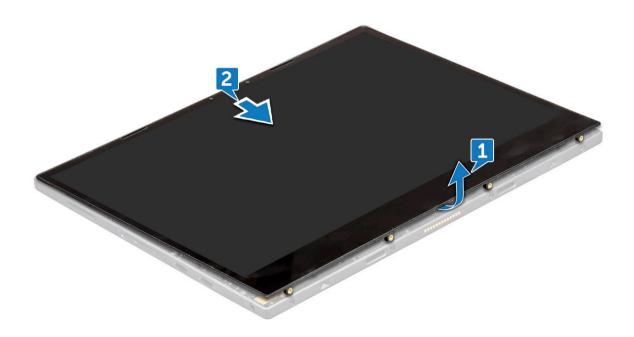
8 Slide the display panel [1], and flip the display panel [2].
