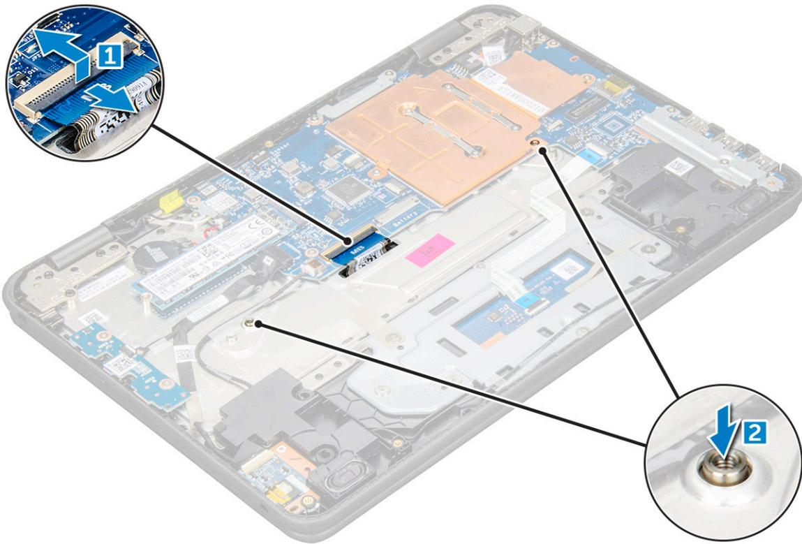
**① | NOTE:** The two release holes for the keyboard are indicated by the "KB" labeling.
