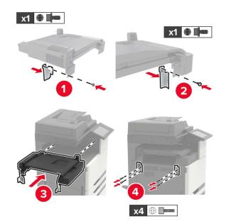
Attach the finisher to the printer.
