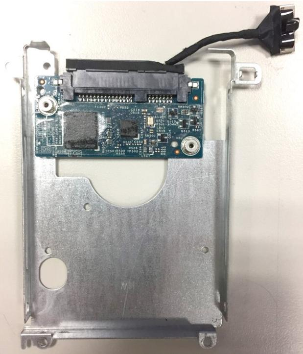
5 Flip the hard drive bracket, remove the screws (M2.0) and take out the eMM card from the bracket.
