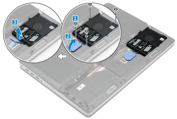
4 Remove the M3.0x3.0 screws that secure the hard drive. Lift the hard drive from the bracket.
