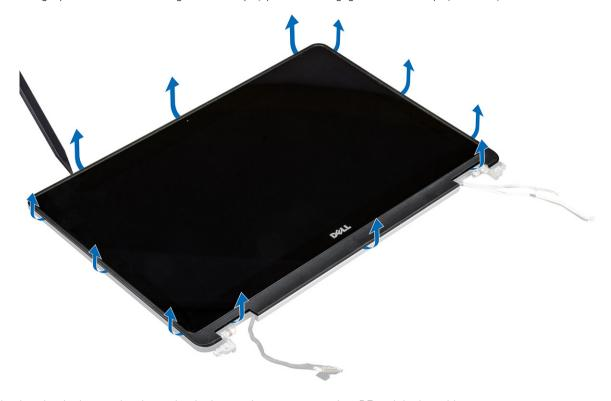
b Lift the display panel and turn the display panel over to access the eDP and display cables.
