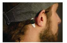
SmartSleep uses dual sensors for highly accurate tracking that is critical to the technology. An adhesive, disposable sensor is used due to the unique placement behind the ear. Each selfadhesive SmartSleep Sensor lasts between 1 and 3 nights of use, depending on factors such as skin conditions and time between usages, when properly applied and stored. Experience the sleep sensing technology of SmartSleep. Headband comes with 30 sensors, replenishments sold separately.
