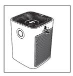
**3** Press the two clips down and pull the pre-filter towards you.
