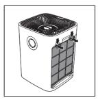
4 Put the unpacked air purification filter back into the appliance.
