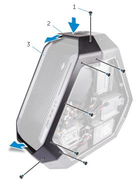
Figure 55. Removing the front-handle bar
