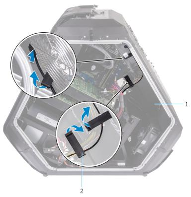
Figure 62. Removing the optical-drive eject-button board cable
