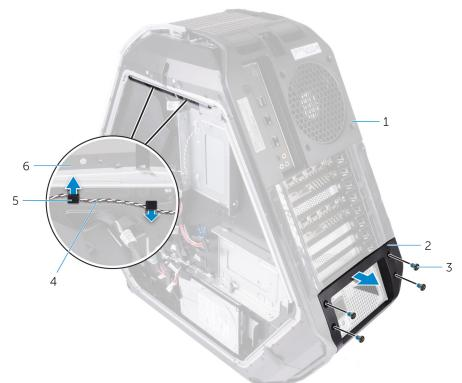
Figure 66. Removing the rear I/O accessibility lighting cable
