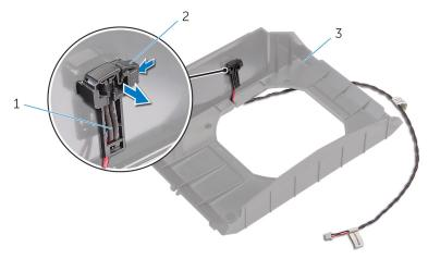
Figure 44. Removing the front-bezel heat-sensor cable
