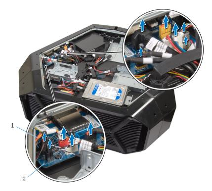
Figure 20. Removing the I/O board
