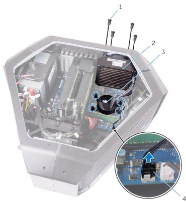
Figure 45. Removing the processor liquid-cooling assembly
