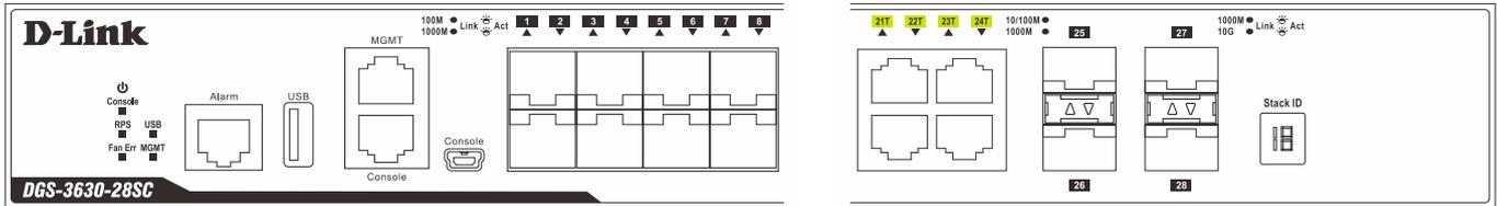
Figure 2-6 LED indicators for the DGS-3630-28SC
