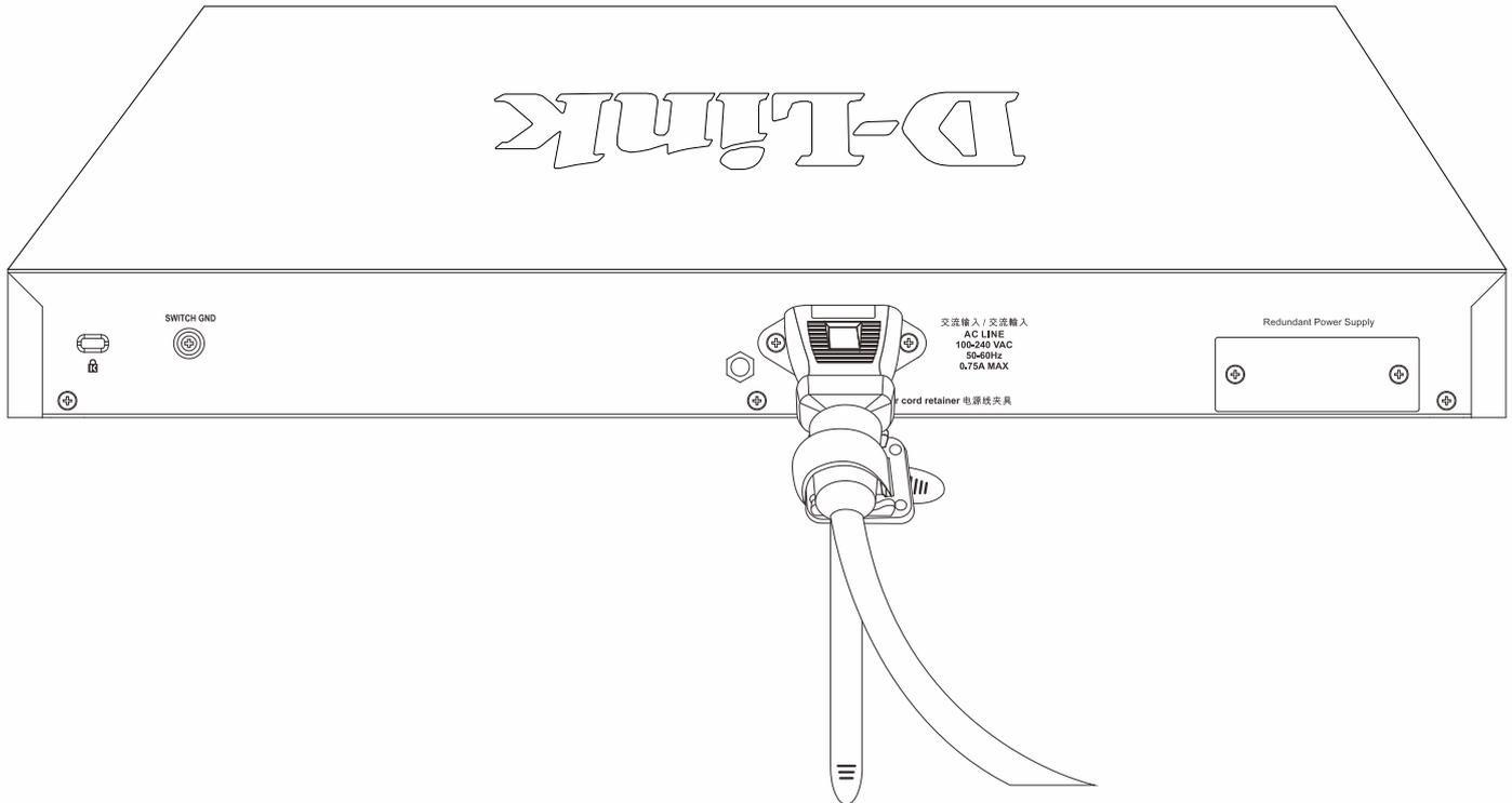
Figure 3-9 Secure the power cord
