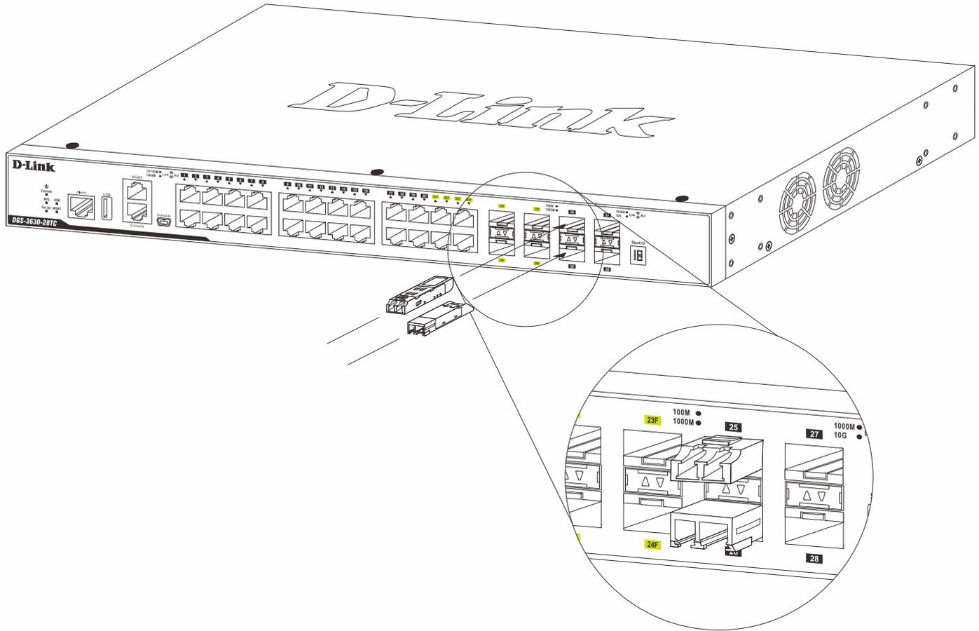
Figure 3-4 Inserting transceivers into the transceiver ports
