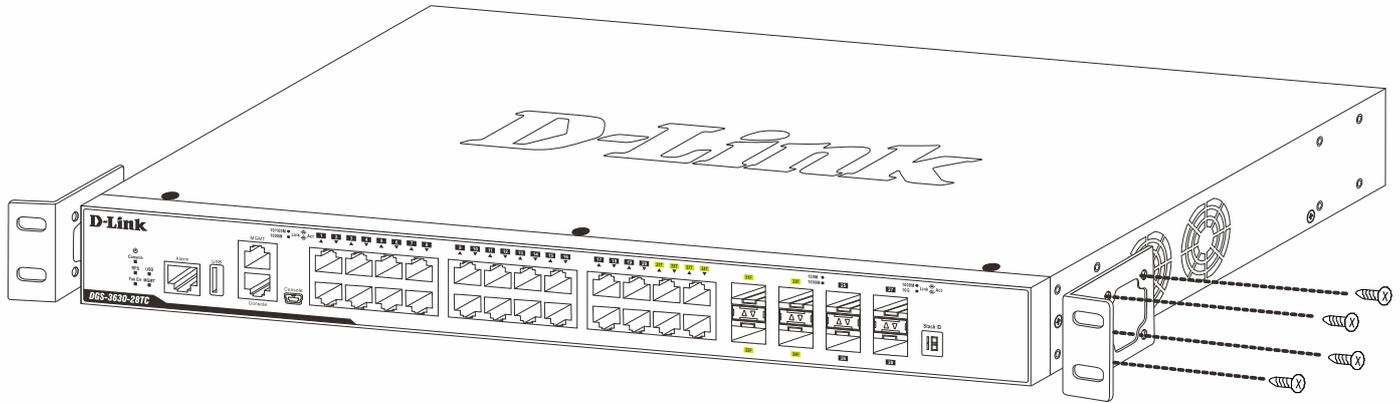
Figure 3-2 Attaching rack-mount brackets to the Switch
