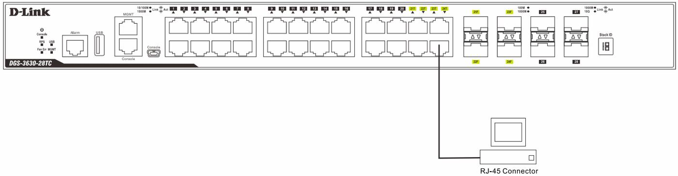
Figure 4-1 Connecting the Switch to an End Node
