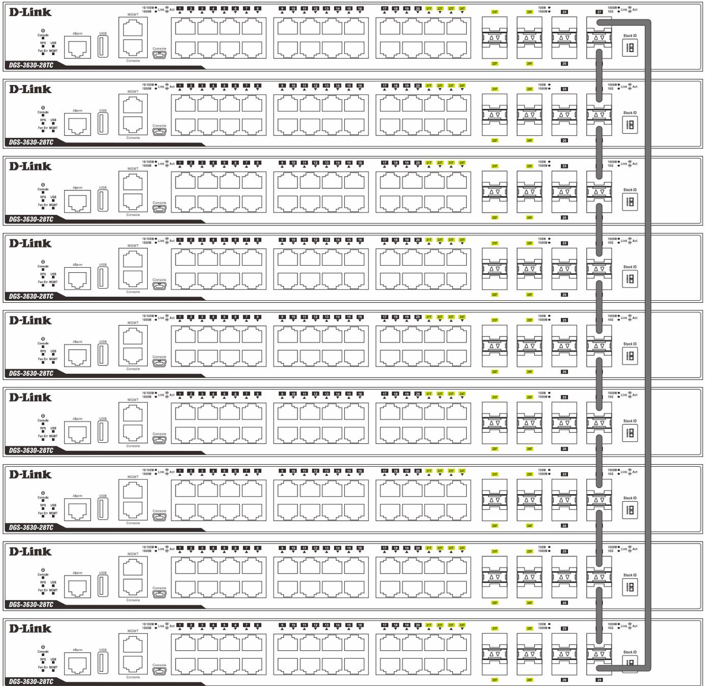
Figure 4-4 Duplex Ring stacking topology (SFP+)
