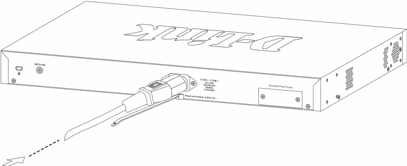
Figure 3-6 Connect the power cord to the Switch
