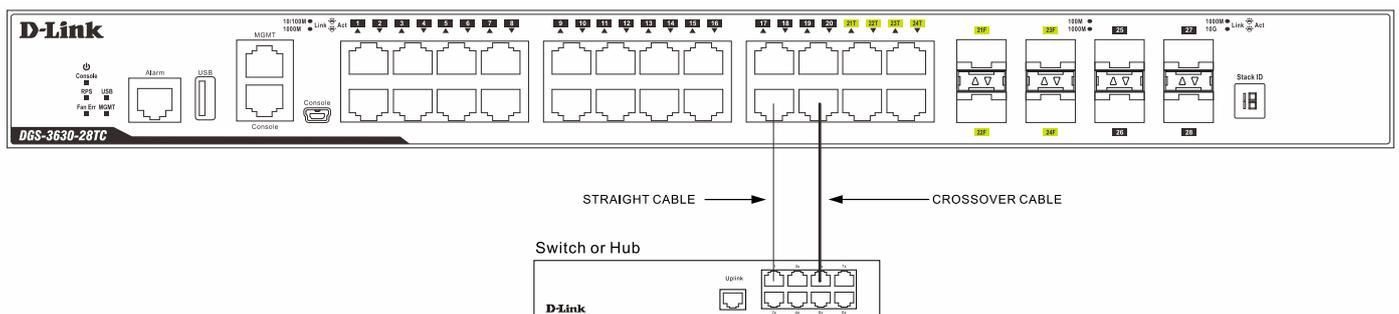
Figure 4-2 Connecting the Switch to another switch/hub
