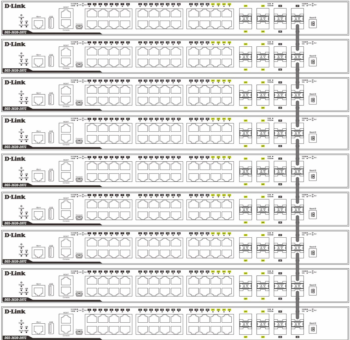
Figure 4-3 Duplex Chain stacking topology (SFP+)
