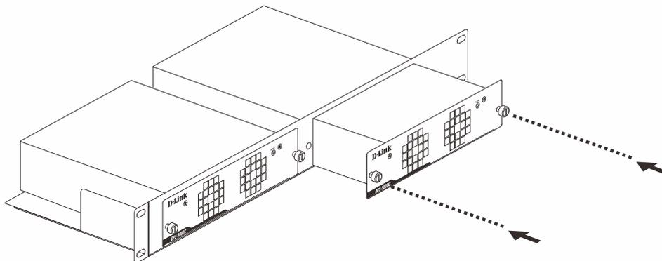
Figure 3–11 Install the DPS-500A in the DPS-800
