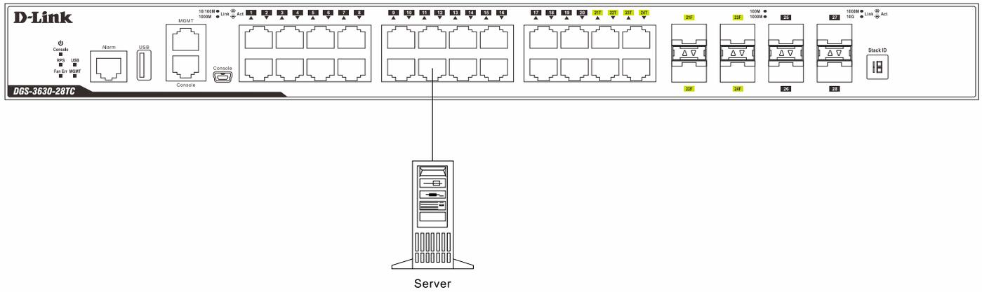
Figure 4-5 Connecting the Switch to a server
