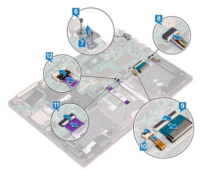
**13** Remove the two screws (M2x2) that secure the system board to the keyboard bracket.
