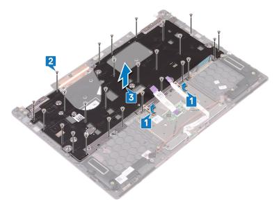
**4** Remove the six screws (M1.2x1.5) that secure the keyboard to the palm-rest assembly.
