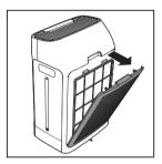
To remove the pre-filter, press the two clips down and pull the filter towards you.
