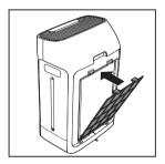
6 To reattach the back cover, mount the panel onto the bottom of the appliance first, and then push the top of the panel against the appliance.
