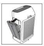
2 Lift the water tray upwards and pull it out horizontally.
