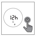
To deactivate the timer function, touch the Timer/Reset button (2) repeatedly until "---" displays on the screen.
