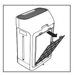
Wash the pre-filter under a running tap. If the pre-filter is very dirty, use a soft brush to brush away the dust.
