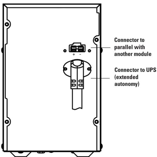
Battery module for models 0.7 and 1 kVA
