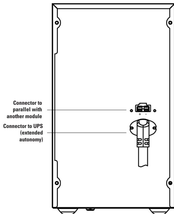
Battery module for models 1.5 and 3 kVA
