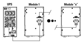
Fig. 11. Connectionamongtheequipmentand"n"batterymodules.
