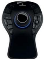
Using the SpaceMouse™ Pro 3D mouse to navigate 3D models or environments is as simple as holding them in your hand. A slight movement of the controller cap delivers easy and precise control. SpaceMouse™ Pro is a companion to the traditional mouse and is operated with the free hand. Your traditional mouse hand is free to select, create and edit.
