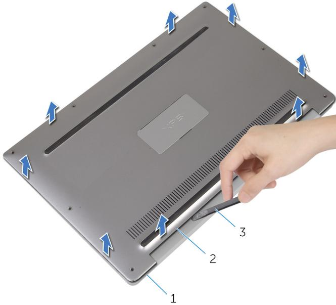
**Figure 2. Removing the base cover**
