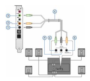
Rear audio connector on the 5 Center/LFE surround out on 1 computer 😂 💽 the speaker Center/LFE surround out on 2 6 Front audio connector on the the computer **\$** speaker Front audio connector on Rear audio connector on the 3 7 the computer (\*\*) speaker 5.1 channel audio cable 4
