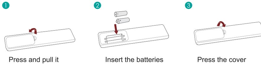
2. Insert two AAA size batteries. Make sure to match the (+) and (-) ends of the batteries with the (+) and (-) ends indicated in the battery compartment.
