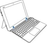
**WARNING!** Ensure to dock your ASUS Tablet on the ASUS Mobile Dock by the orientation shown above. Incorrect docking may cause damage to your device.
