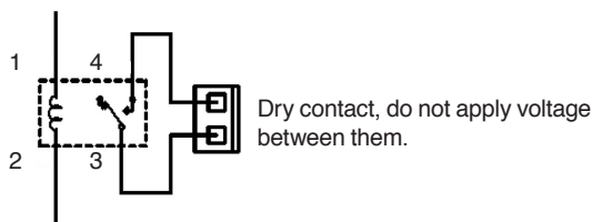
Fig. 15. Dry contact "Dry_out".
