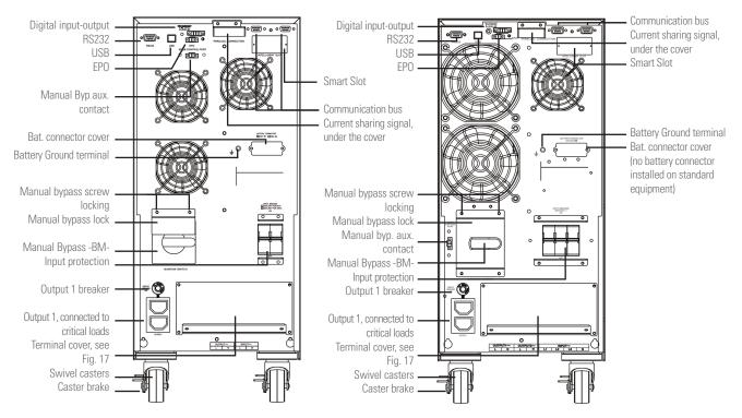
Standard and B1, from 4 to 10 kVA. Single phase input and output.
