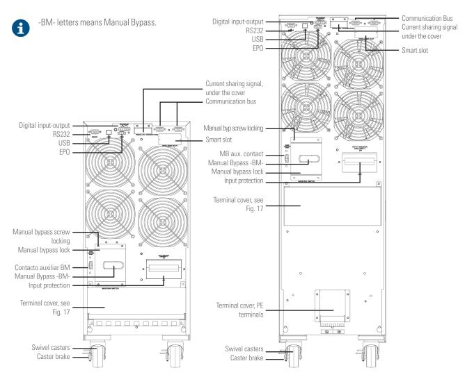
B1, from 15 and 20 kVA. Three phase input and single phase output.
