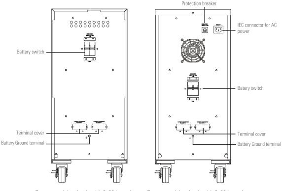
Battery module, size 1, with 2x20 batteries and 50 A protection.
