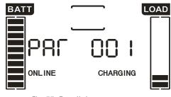
Fig. 55. Parallel system screen.
