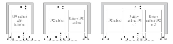
Fig. 14. Minimum distances for a correct UPS cooling.
