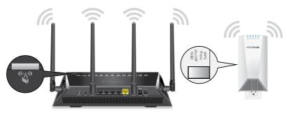
Press the WPS/Power button on the extender for less than five seconds.
