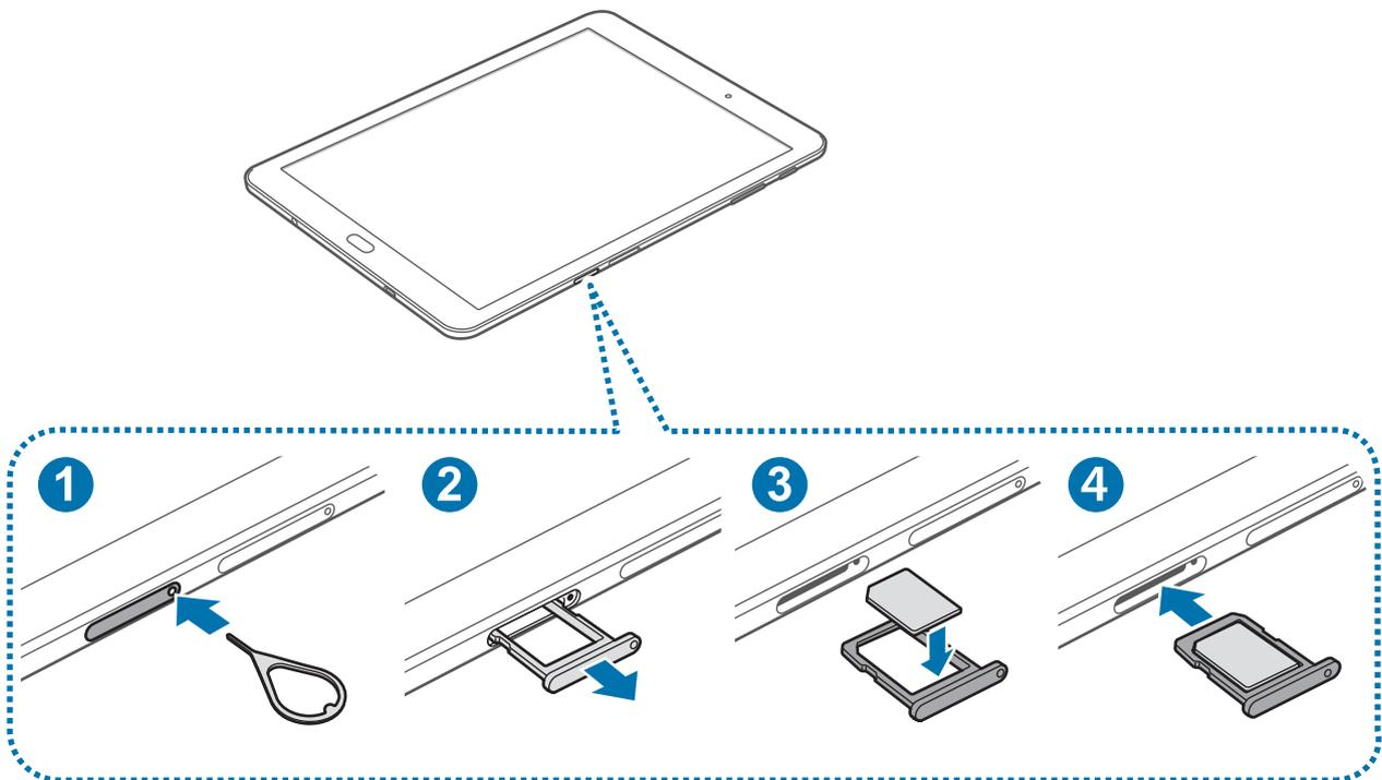
**1** Insert the ejection pin into the hole on the SIM card tray to loosen the tray.
