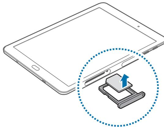
4 Insert the SIM card tray back into the SIM card tray slot.
