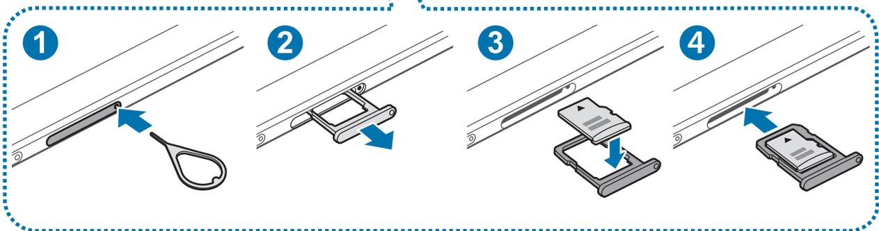
1 Insert the ejection pin into the hole on the memory card tray to loosen the tray.
