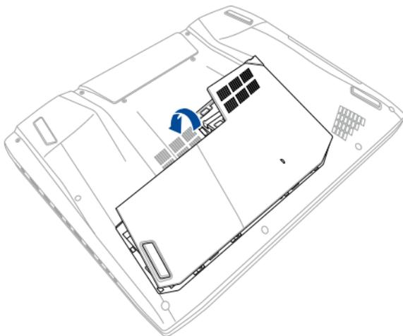
P. Reattach and tighten the screw that you removed earlier.
