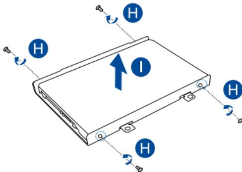
To remove an HDD attached to the HDD bay:
