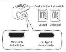
1 Slide the lock switch to the ∩ position and remove the device holder from the Gear VR.
