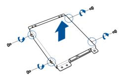
7. To install a new HDD/SSD, secure the HDD/SSD to the bracket using four (4) screws.
