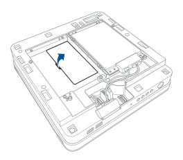
4. Align and insert the memory module into the slot (A) and press it down (B) until it is securely seated in place. Repeat the same steps to install the other memory module.
