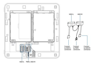
9. Connect the cable to the HDD/SSD, then align the bracket to the HDD/SSD compartment of your VivoMini and secure the bracket with the screws previously removed.
