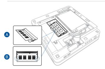
**IMPORTANT!** Always install into the lower slot first.
