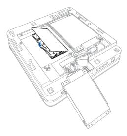
6. Align the HDD1L bracket and secure it using the screws removed previously.
