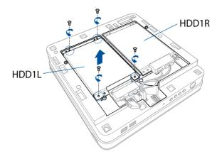
6. (optional) To upgrade your HDD/SDD, first remove the four (4) screws on the bracket, then remove the bracket.
