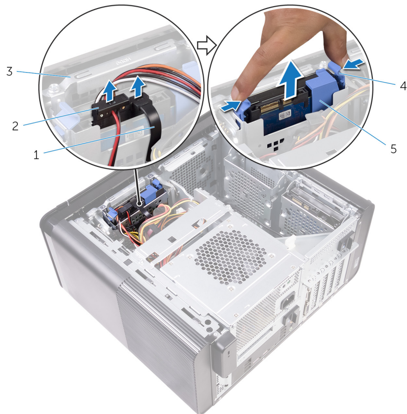
Figure 13. Removing the hard-drive assembly
