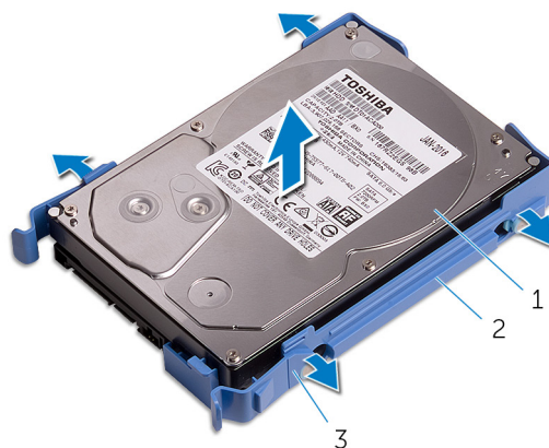
Figure 14. Removing the hard drive from the bracket
