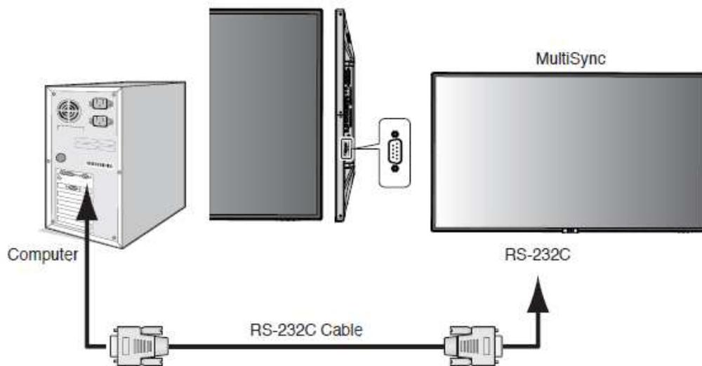
(Please refer "Controlling the LCD monitor via RS-232C Remote control" on User's manual.)
