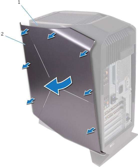
Figure 2. Removing the right-side cover
