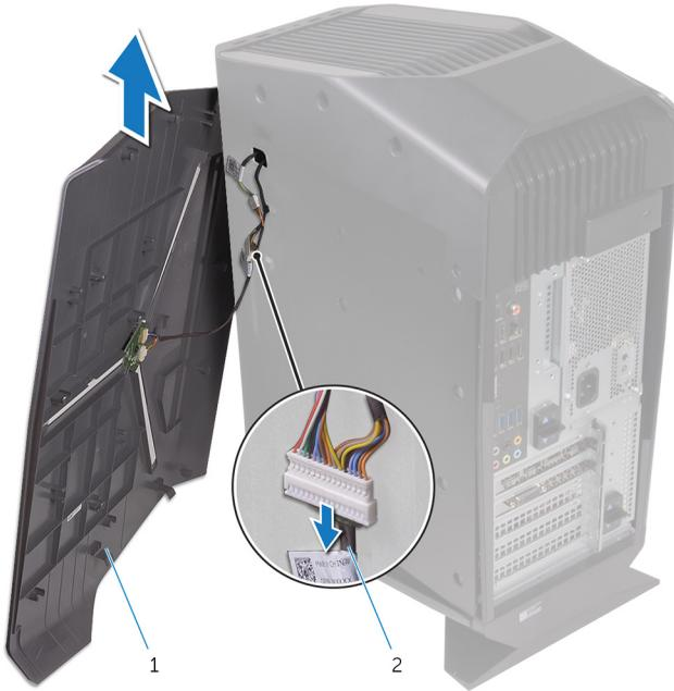
**Figure 3. Removing the right-side cover**
