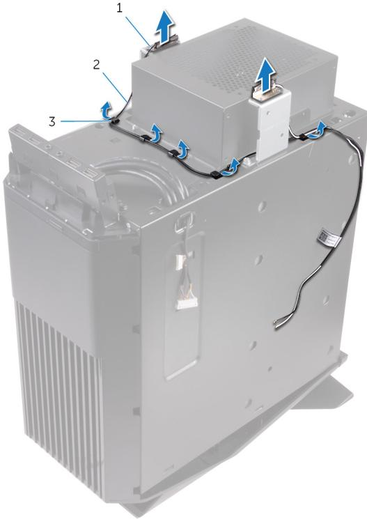
**Figure 32. Removing the antenna cables**
