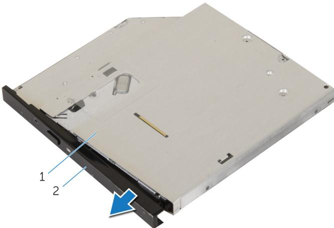
**Figure 40. Removing the optical drive**
