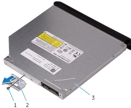
**Figure 39. Removing the optical drive**
