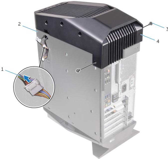
**Figure 6. Removing the top cover**
