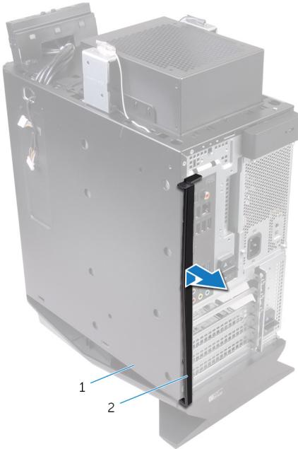
**Figure 45. Removing the rear trim cover**
