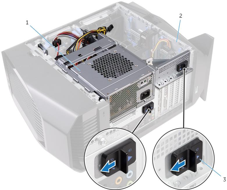
**Figure 18. Sliding the power-supply unit cage release latches**
