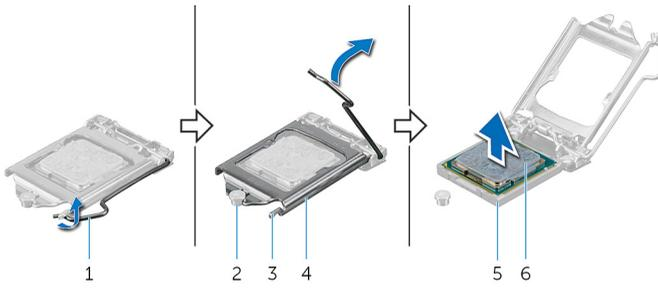
**Figure 27. Removing the processor**
