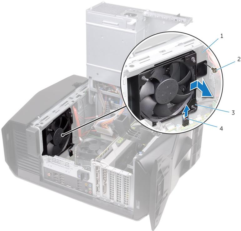
**Figure 35. Removing the top-chassis fan**
