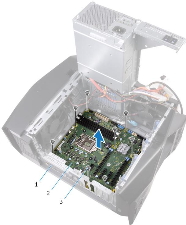
**Figure 47. Removing the system board**
