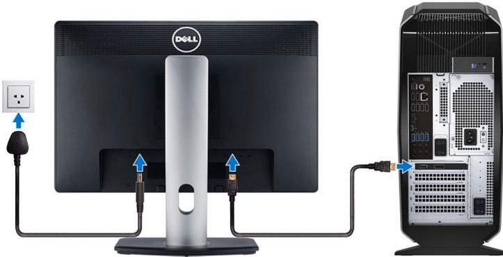
**NOTE:** The DisplayPort on the back panel of your computer is covered. Connect the display to the discrete graphics card of your computer.
