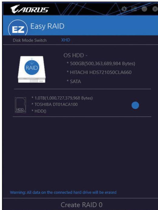
(Note 1) The XHD utility only supports the SATA connectors controlled by the Intel® Chipset.
