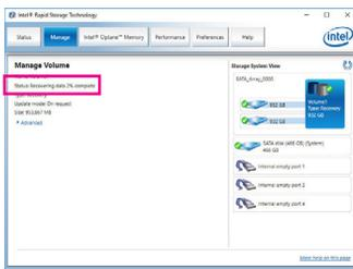
The **Status** item on the left of the screen displays the recovering status. After the recovery volume is completed, the **Status** will display as **Normal**.
