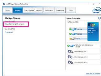
The **Status** item on the left of the screen displays the rebuild progress. After the RAID 1 volume rebuilding, the **Status** will display as **Normal**.
