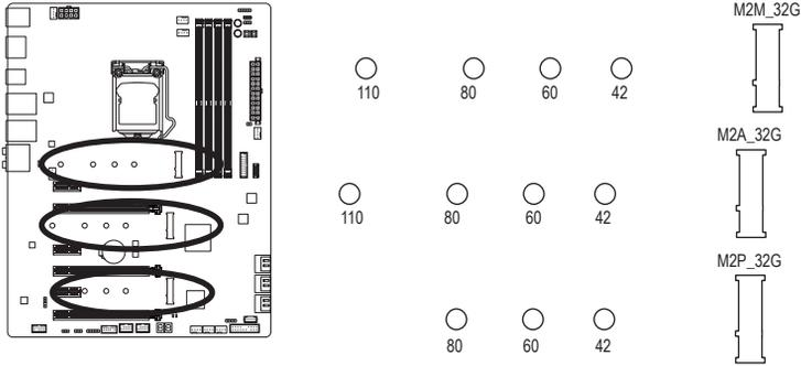
Follow the steps below to correctly install an M.2 SSD in the M.2 connector.
