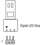
Connect your digital LED strip to the header. There are 12V and 5V digital LED strips. Be sure to verify the voltage requirements of your digital LED strips and set the DLED\_V\_SW1 and DLED\_V\_SW2 jumpers accordingly. The power pin (marked with a triangle on the plug) of the LED strip must be connected to Pin 1 of the digital LED strip header. Incorrect connection may lead to the damage of the LED strip.
