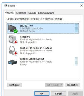
For example, in Windows 10, right-click the speaker icon in the notification area and click **Playback devices**. On the **Playback** tab, set **Intel(R) Display Audio** to the default playback device.
