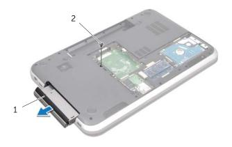
1 optical-drive assembly 2 screw
