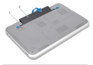
1 battery release latches (2) 2 battery
