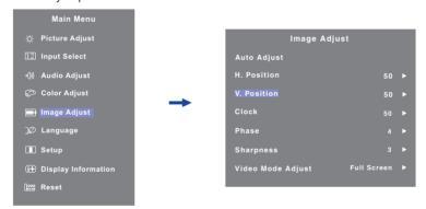
Then, use the ◀ / ▶ Buttons to change the vertical position settings. The vertical position of the overall display should be changing accordingly while you are doing this.
