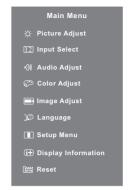
For example, to correct for vertical position, select Menu item of Image Adjust and then press the ENTER Button. Then, select V.Position by using the ◀ / ▶ Buttons. An adjustment page appears after you press the ENTER Button.
