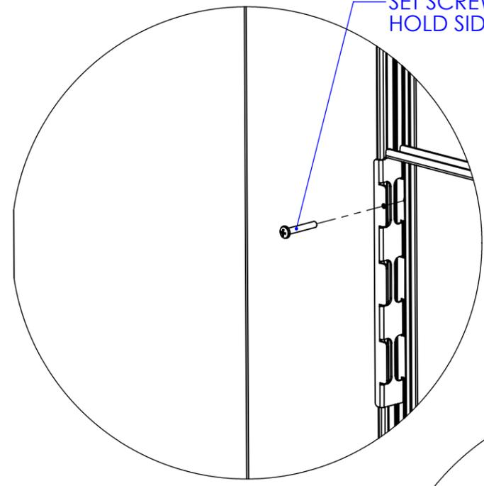
SET SCREW, TIGHTEN AS REQUIRED TO HOLD SIDE COVER MATERIAL
