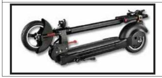
1. Locate and press down on the Frame Folding Switch.
