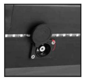
Using the enclosed cable, attach the charging cable to your eKick 10 pro by aligning the cable pins. Plug the other end into a grounded wall outlet.
