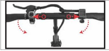
2. Twist the Steering Column Height Adjuster counterclockwise to loosen it.
