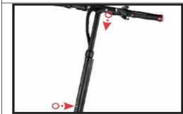
4. Adjust the steering column lock so that it can not move.
