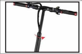
3. Locate the Steering Column Lock and press down to loosen it. With the Steering Column Lock pushed down, push the Steering Column down to its lowest height. The Steering Column Lock will click and lock in place.
