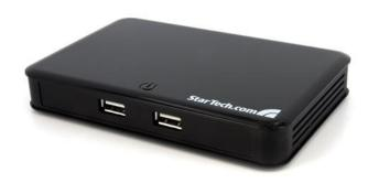
The USB2VGADVI USB to VGA/DVI-I adapter turns a USB 2.0 port into both a DVI-I and VGA video output port. Similar to our existing <u>USB video adapters</u>, the USB2VGADVI offers a convenient and cost-effective solution for adding multiple monitors to your computer without having to open the computer case for typical video card installation.
