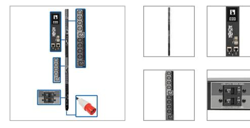
28.8kW 3-phase PDU with multi-function touchscreen LCD distributes, monitors and manages AC power. Built-in Java-free network interface helps you remotely monitor load levels to prevent overloads that cause downtime.
