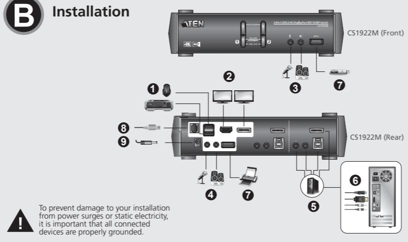
To prevent damage to your installation from power surges or static electricity, it is important that all connected devices are properly grounded.
