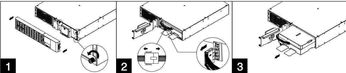
1. Remove faceplate and unscrew the thumbscrews on toolless battery access door and then open the door. Note: Thumbscrews are designed fixed on the door, do not remove them from the metal cover.
