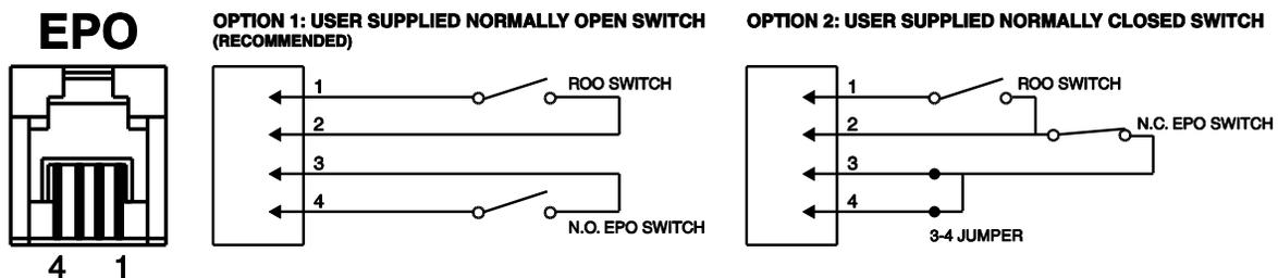
3. After wiring, make sure the external EPO/ROO switch is not activated to enable UPS output.
