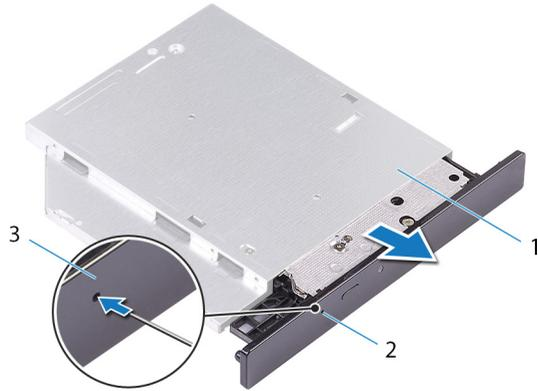
**Figure 8. Removing the optical-drive bezel**
