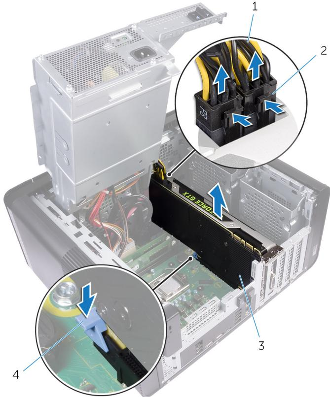
**Figure 23. Removing the power cable**
