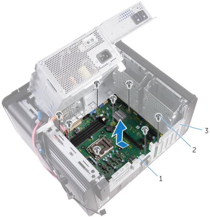
**Figure 42. Removing the system board**
