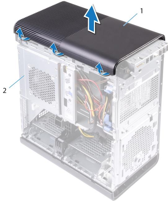
**Figure 10. Removing the top cover**
