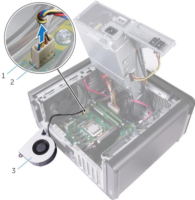
**Figure 31. Removing the blower cable**
