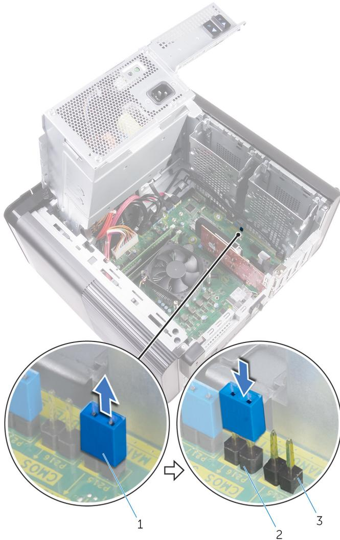
**Figure 43. Clearing the CMOS**
