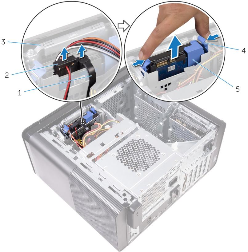
**Figure 13. Removing the hard-drive assembly**
