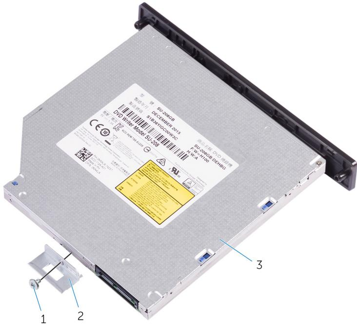
**Figure 7. Removing the optical drive**
