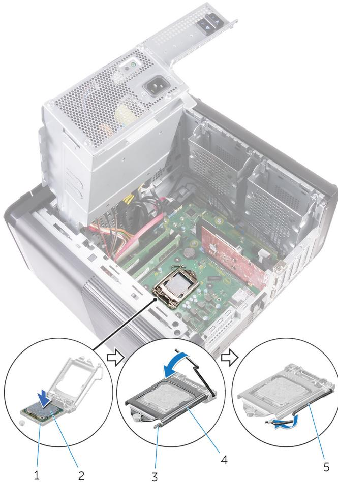
**Figure 37. Replacing processor**
