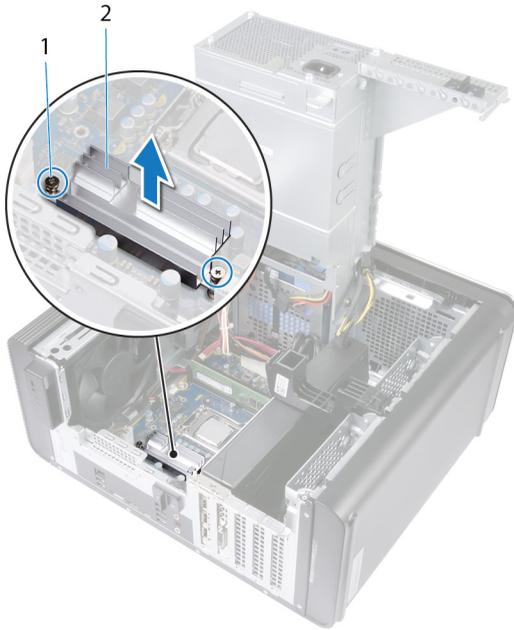
**Figure 32. Removing the VR heat sink**
