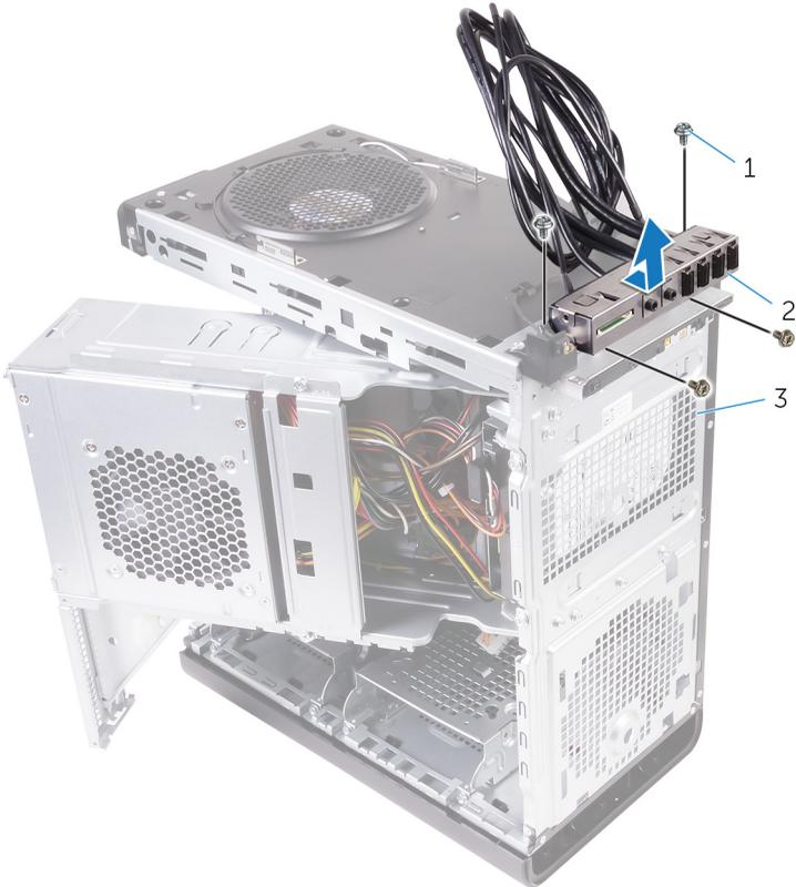
**Figure 28. Removing the USB panel**
