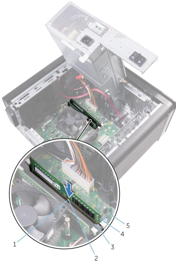
**Figure 25. Replacing the memory module**
