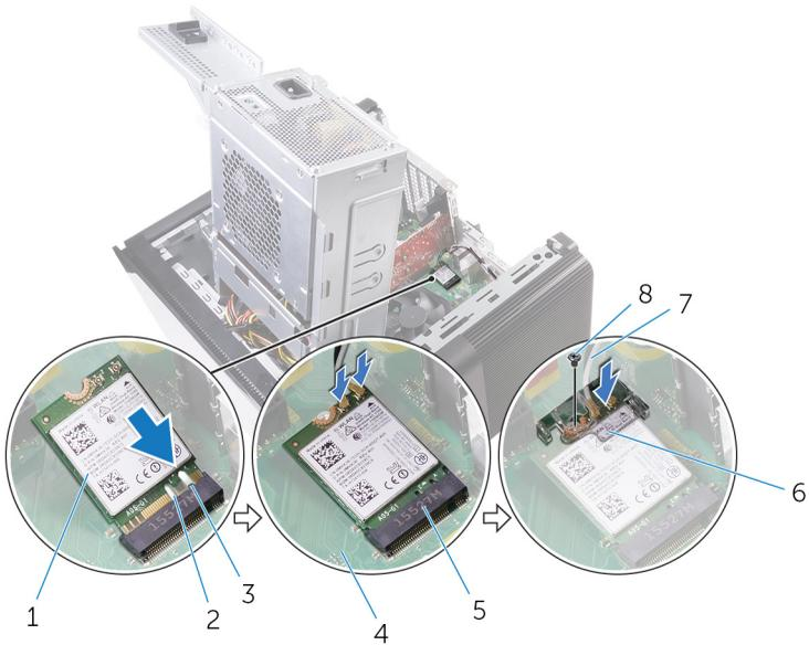
**Figure 39. Replacing the wireless card**
