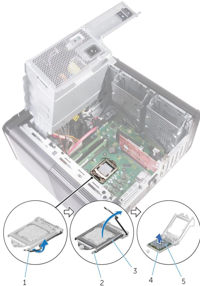
**Figure 36. Removing processor**
