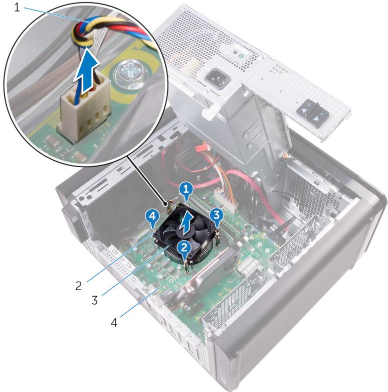
**Figure 33. Removing the processor fan and heat sink**
