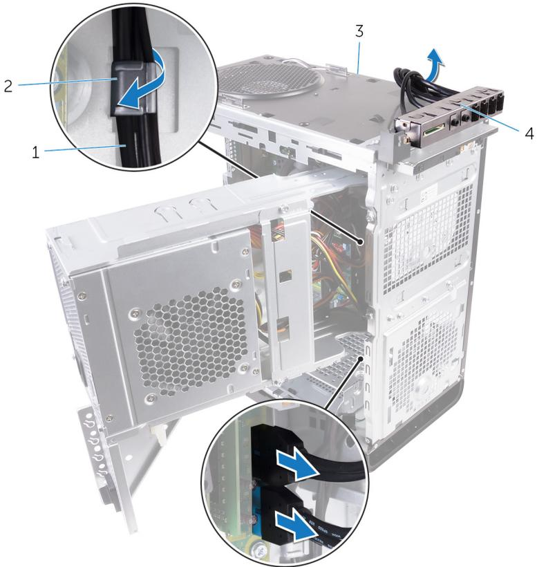
**Figure 27. Disconnecting the cables**
