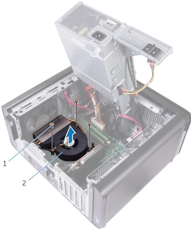
**Figure 29. Removing the blower**
