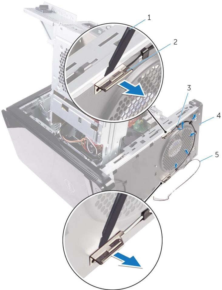
**Figure 41. Removing the antenna**
