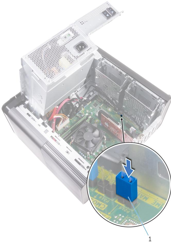
**Figure 45. Clearing the password**
