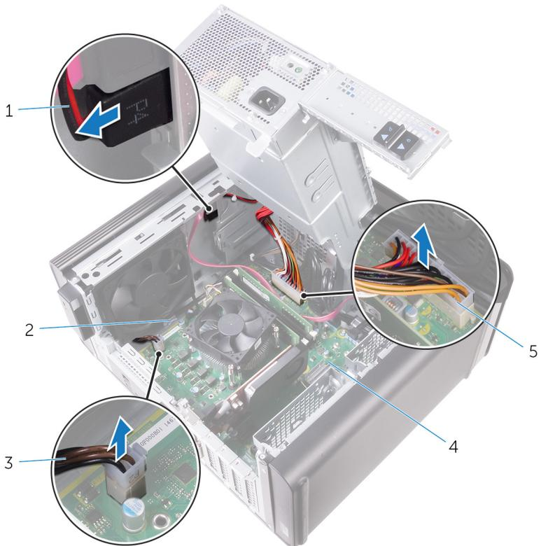
**Figure 18. Disconnecting cables**
