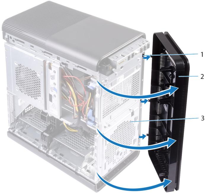
**Figure 4. Removing the front bezel**
