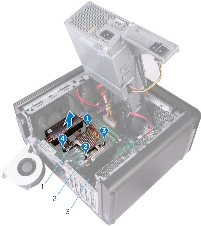
**Figure 30. Removing the captive screws**
