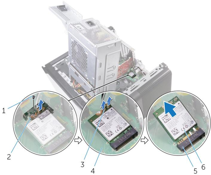
**Figure 38. Removing the wireless card**
