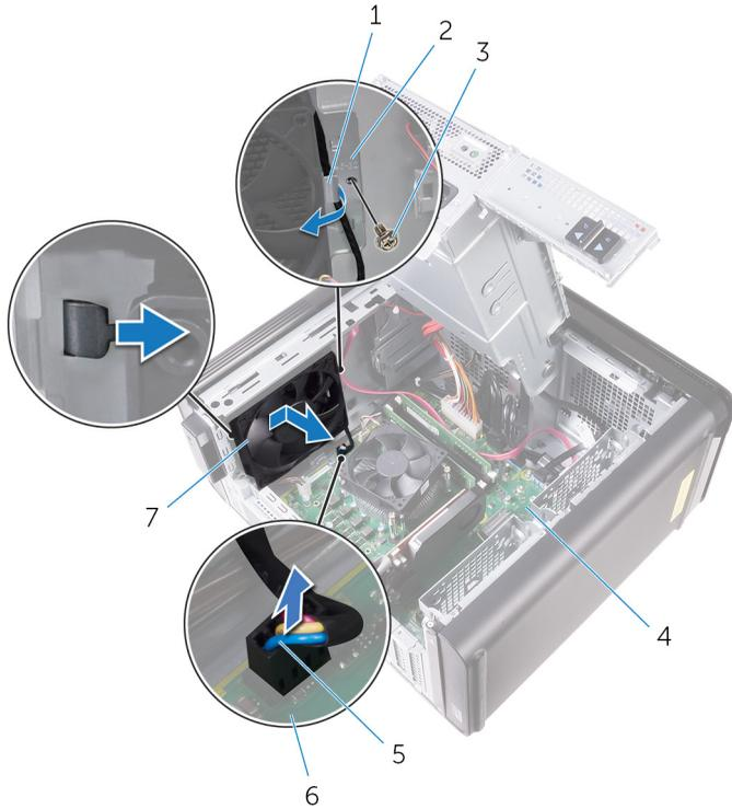
**Figure 34. Removing the chassis fan**
