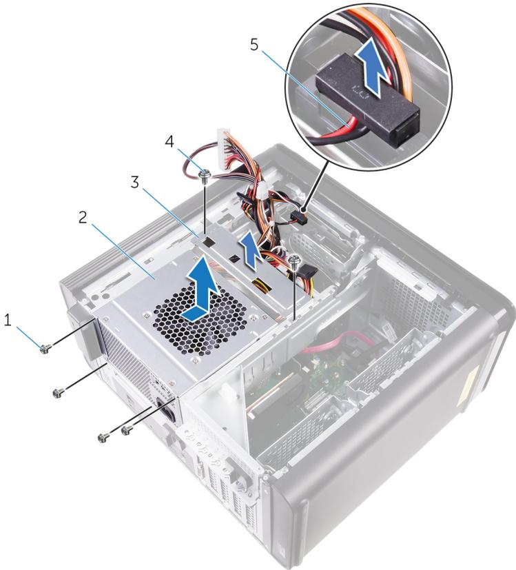
**Figure 19. Removing the power supply unit**
