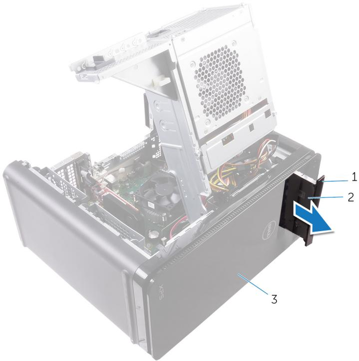
**Figure 6. Removing the optical drive**
