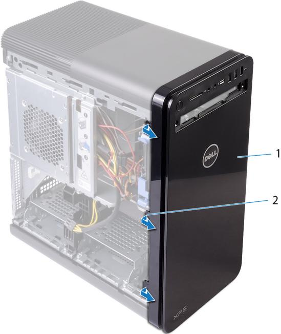
**Figure 3. Removing the front bezel**
