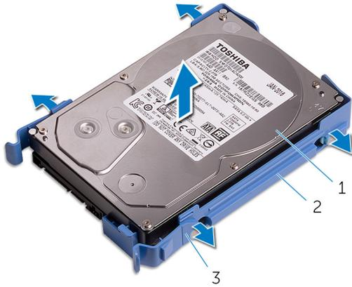
**Figure 14. Removing the hard drive from the bracket**
