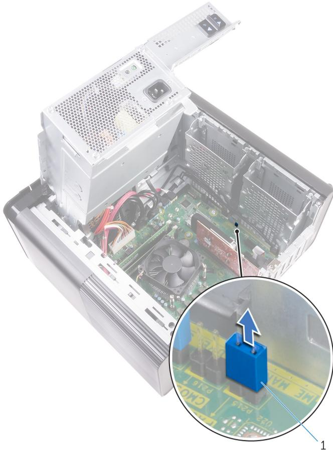
**Figure 44. Removing the jumper plug**
