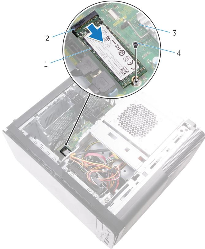
**Figure 15. Removing the solid-state drive**
