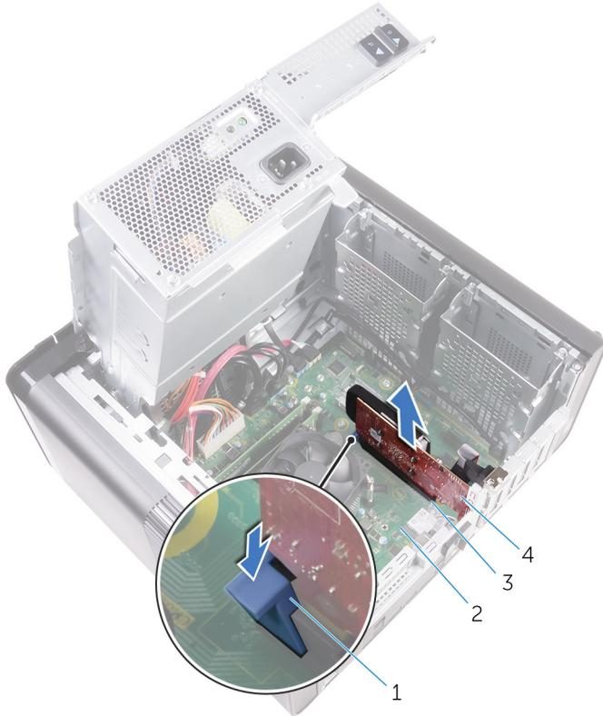
**Figure 21. Removing the graphics card**
