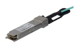
The QSFP40GAO15M is an MSA compliant optical quad small form-factor pluggable (QSFP+) cable that is designed, programmed and tested to work with 40 GbE compatible switches and routers. This AOC QSFP+ cable supports 40 Gigabit Ethernet applications ( $4 \times 10$ GbE) connected through QSFP+ ports. It is a low-power, low-latency cable that is hot-swappable, making upgrades and replacements seamless by minimizing network disruptions.
