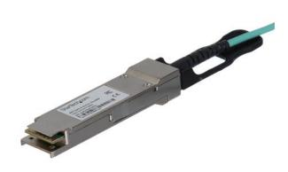
The QSFP40GAO7M is an MSA compliant optical quad small form-factor pluggable (QSFP+) cable that is designed, programmed and tested to work with 40 GbE compatible switches and routers. This AOC QSFP+ cable supports 40 Gigabit Ethernet applications ( $4 \times 10$ GbE) connected through QSFP+ ports. It is a low-power, low-latency cable that is hot-swappable, making upgrades and replacements seamless by minimizing network disruptions.
