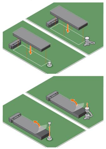
c Place the M.2 Intel optane memory module into the slot on the thermal pad.
