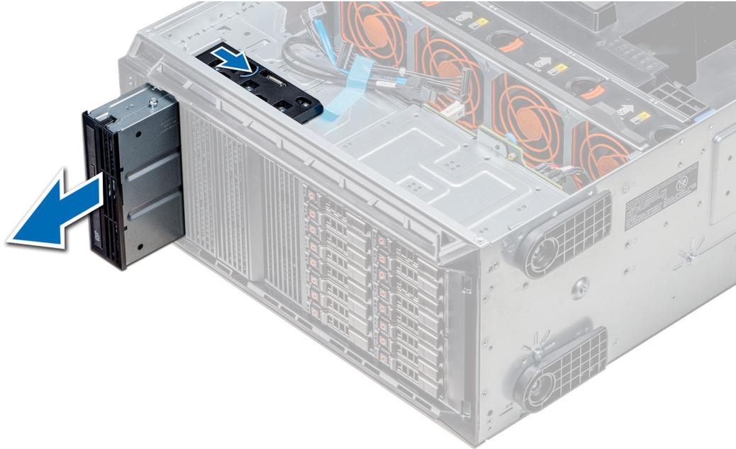
**Figure 50. Removing the optical drive cage or tape drive**
