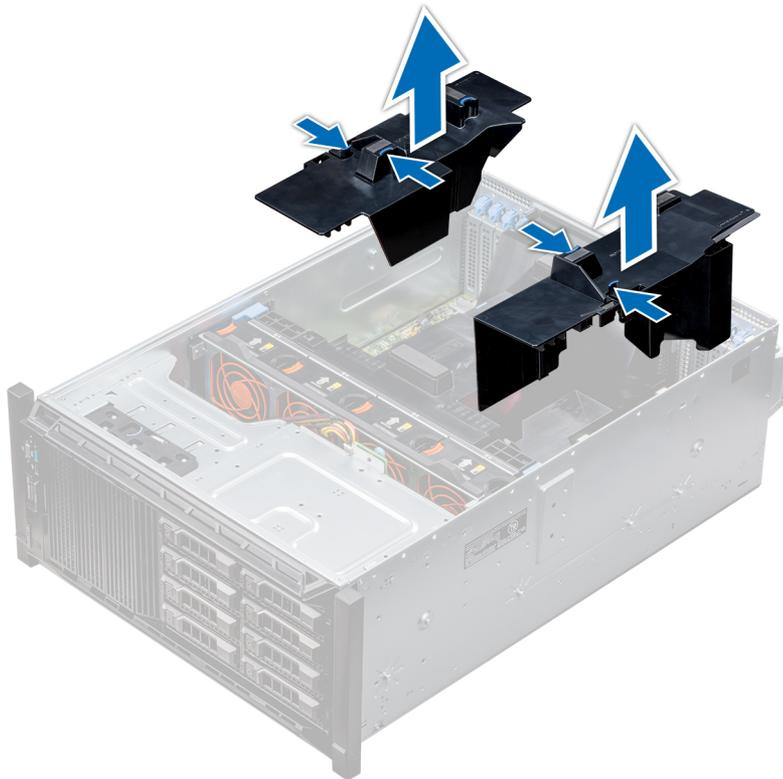
**Figure 36. Removing the optional GPU air shrouds**
