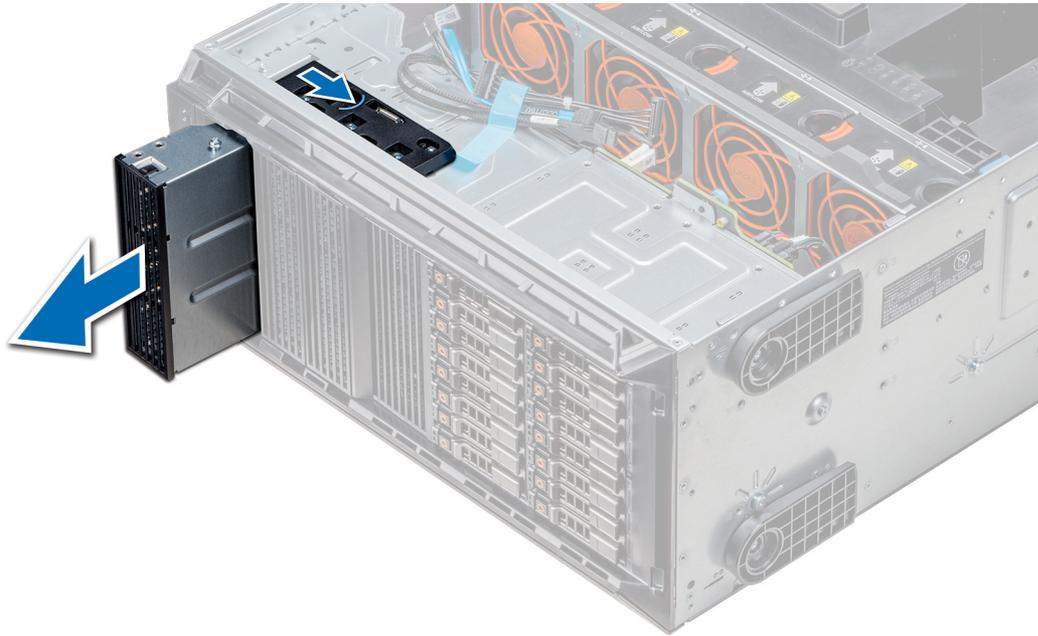
**Figure 48. Removing the optical drive or tape drive**
