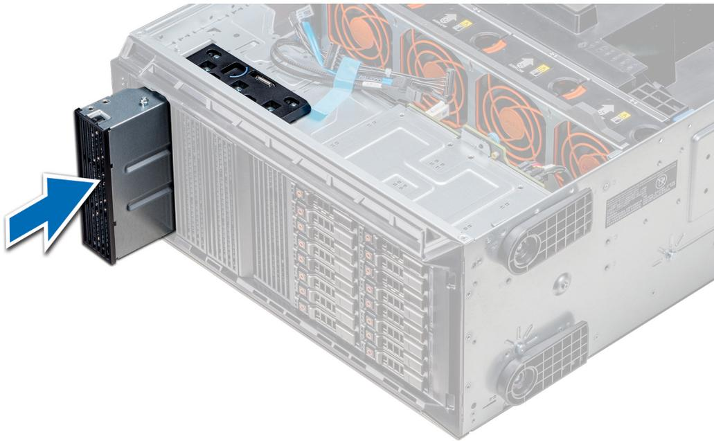
Figure 49. Installing the optical or tape drive blank
