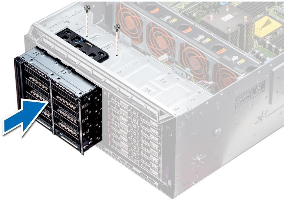
**Figure 47. Installing a NVMe drive bay or flex bay**
