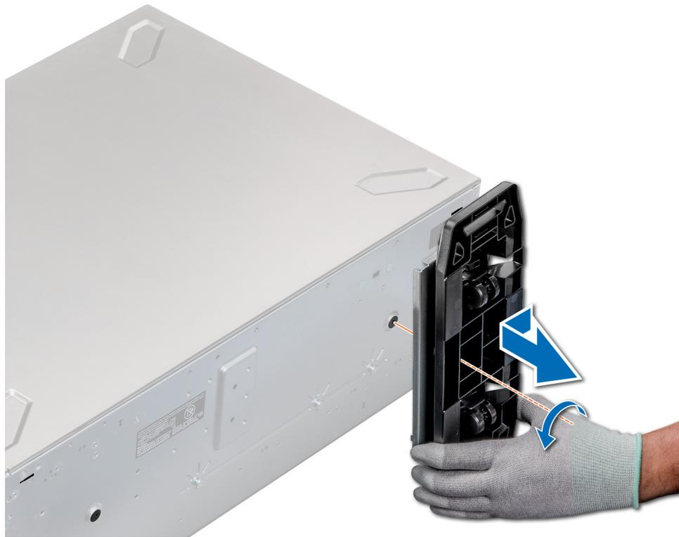
**Figure 19. Removing caster wheels**
