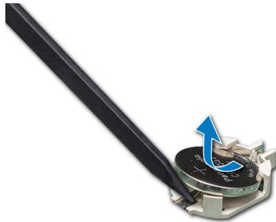
**Figure 89. Removing the system battery**
