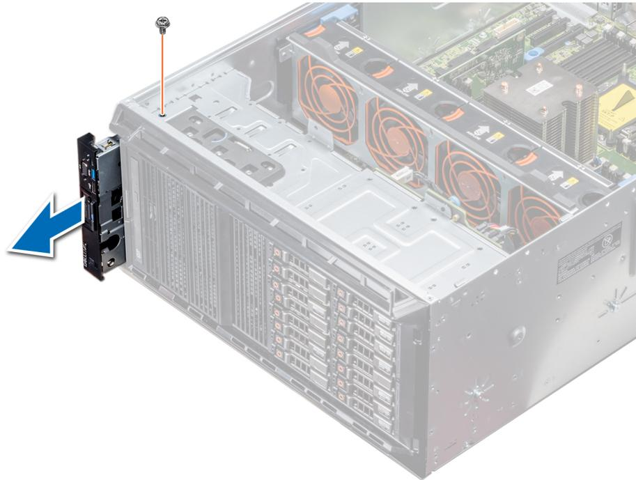
**Figure 101. Removing the control panel assembly**
