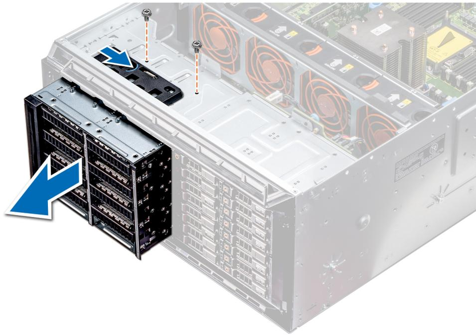
**Figure 46. Removing a NVMe drive bay or flex bay**
