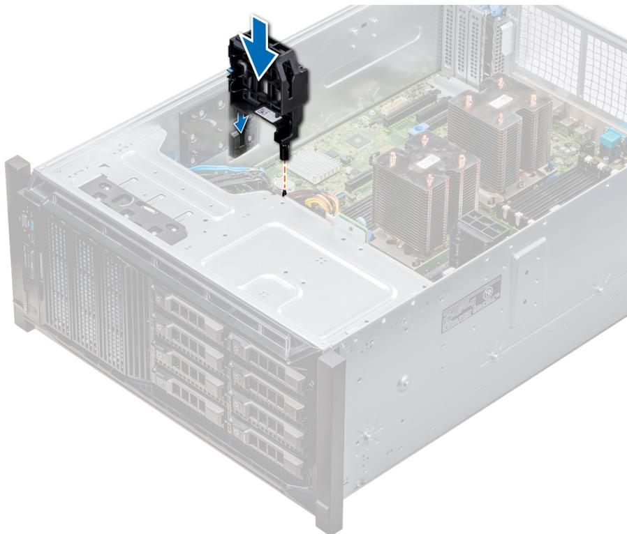
**Figure 68. Installing the optional GPU card holder**
