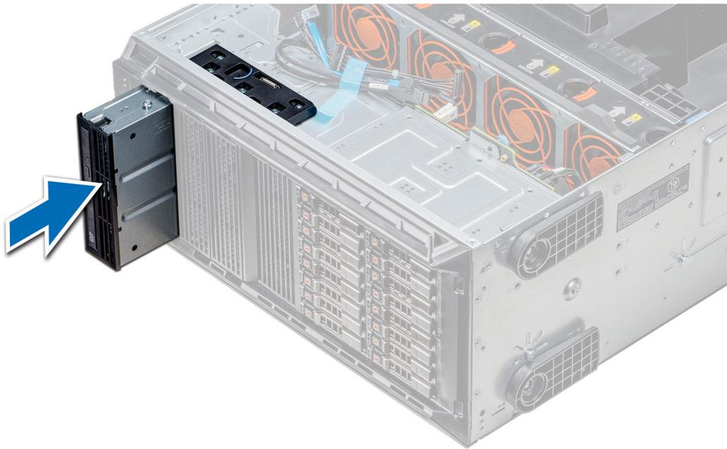
**Figure 51. Installing the optical drive cage or tape drive**
