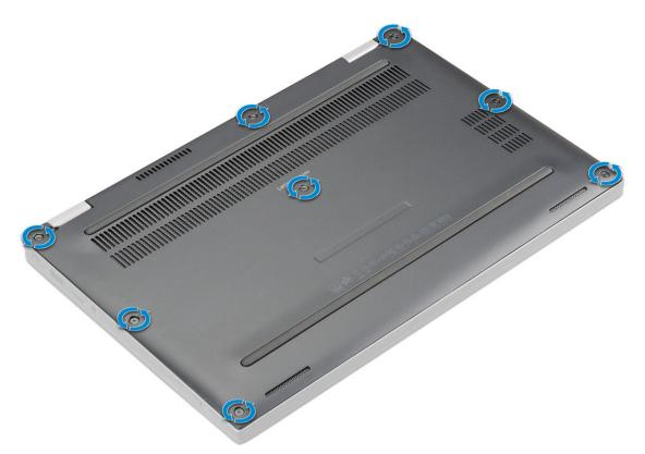
3 Use a plastic scribe to pry the base cover starting from the hinges at the top edge of the base cover and lift it from the computer.
