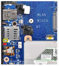
2 Slide the dummy SIM card tray out of the system.
